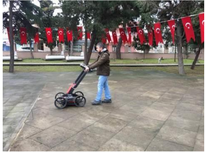
Figure 4. HDR-PRO 450 MHz antenna ground-penetrating radar device
